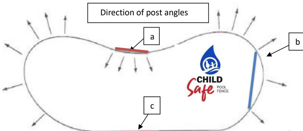
The holes on a line are made perfectly vertical. Use a level on the top for more accuracy. To lean the post, you must make the hole at a certain angle.
