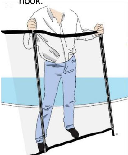
We recommend starting by positioning the gate and then installing the fence. Make sure that the screws on the posts are on the outside of the pool, as in the picture.
